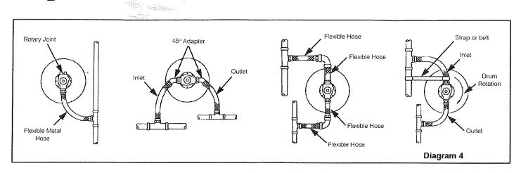
**DEUBLIN** Rotary Unions can usually be easily installed. By following the instructions outlined here, the full potential of the rotary joint for long, trouble-free service will be assured.
